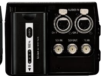
Rear: Battery and Terminal
