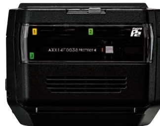
Front: Card slot and Speaker
