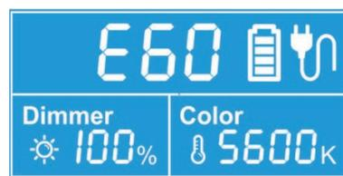
LCD screen displays dimmer, color temperature value, and remaining battery status. Pressing the knobs can switch to quick adjusting mode.
