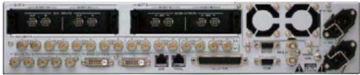
AV-HS450 Rear Panel Interfaces (Mainframe)
