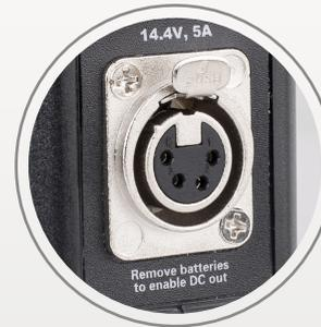
AC-DC adapting output via 4-pin XLR female connector. Offer DC **14.4V, 5A, 72W** output.
